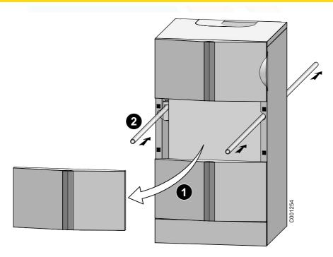
The boiler can be lifted by using 2 tubes Ø3/4" placed as shown in the view.
