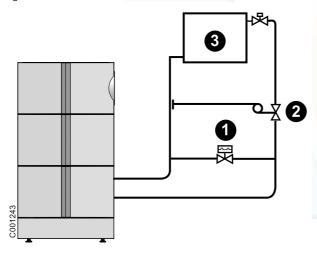
Poor adjustment of the differential valve may cause a continuous increase in the return of water to the boiler.
