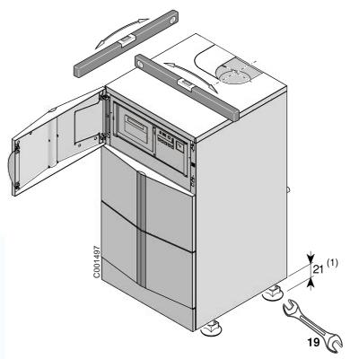
Level the boiler by turning the adjustable feet. To adjust, take the load off the foot using a lever.
