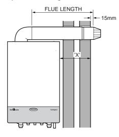
RHS FLUE LENGTH = 'X' + 254mm LHS FLUE LENGTH = 'X' + 10mm
