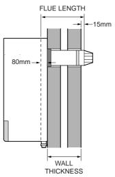
REAR FLUE LENGTH = WALL + 95mm
