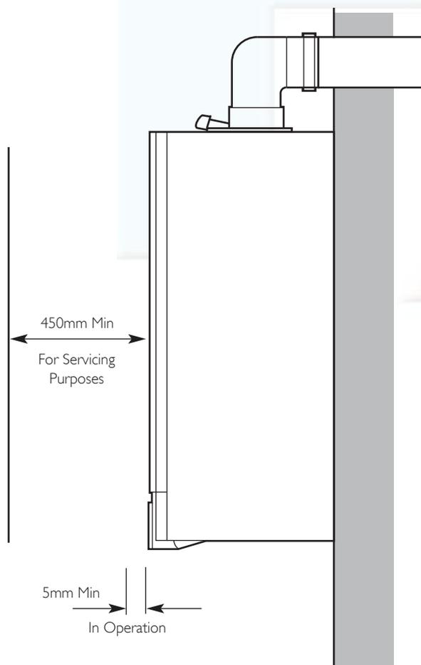
7. If your boiler is installed in a compartment, do not use it for storage purposes. Do not obstruct any purpose provided ventilation openings.
