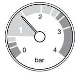
**Central Heating System Pressure** - The normal operating water pressure is between 1 and 2.0 bar. If the pressure exceeds 3 bar the safety pressure valve will operate and a fault is indicated. Contact your Installer.
